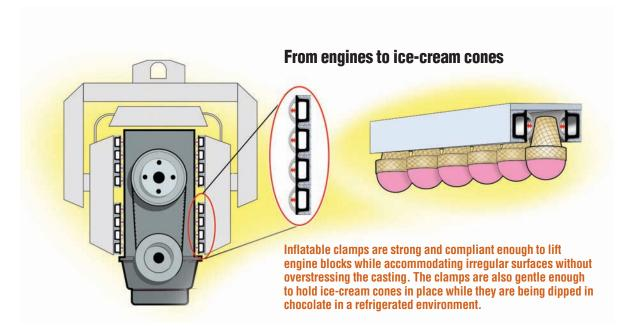
the bulb portion inflates and moves outward. This is the profile used in most conveyor stops and part positioners. The top surface can have a gripping surface that ensures contact despite grit.
