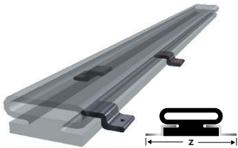
Z-CLIP Stainless steel clips screwed down at defined intervals. Seal is then snaked between clips.
